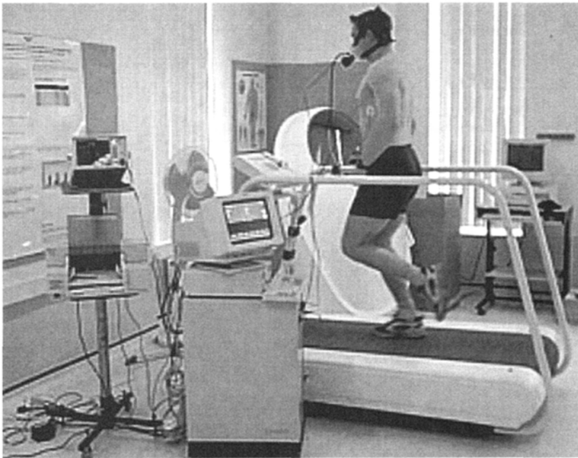
Figure 6.3 A subject running on a motorized treadmill, with expired air analysis through a face mask (Hans Rudolph Inc., KS, USA) connected to an on-line automated breath-by-breath gas analysis system (Oxycon Champion, Mijnhardt, Bunnik, Netherlands; Jaeger, Hoechberg, Germany) and a three-lead ECG through an ECG Oscillograph (CR7 Cardiorater, Cardiac Recorders, Enfield, UK).
